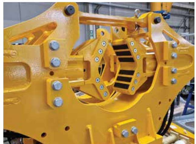
▲ Open face area to allow for larger augers (position 6)
