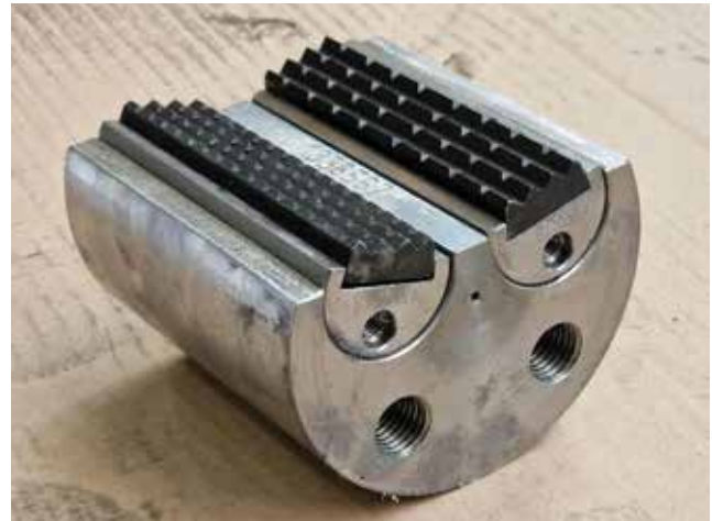
▲ Jaw inserts (position 4) made from carbonated high alloyed steel.
